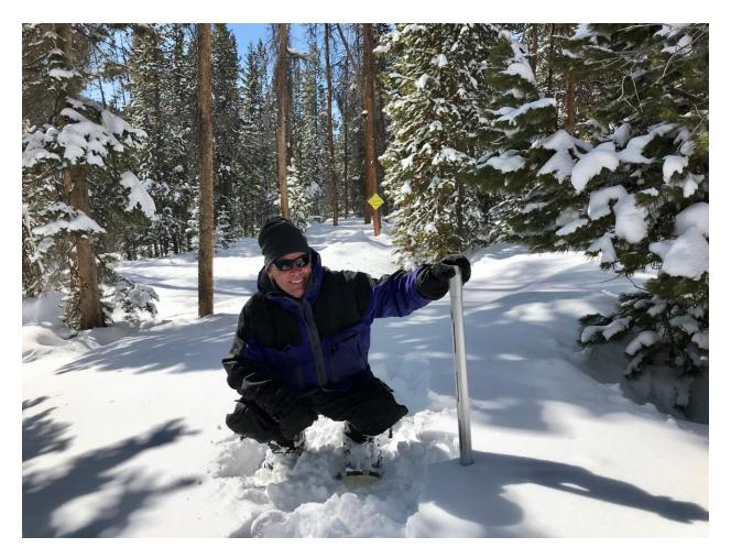
Mark Volt measures near record snow depth and water content at the Gore Pass snow course during the March 1st. snow survey. 52" of snow and 14.1" of water. The only higher snow measured on Gore Pass for March 1st. was in 1962. The Gore Pass snow course has been read since 1951.
